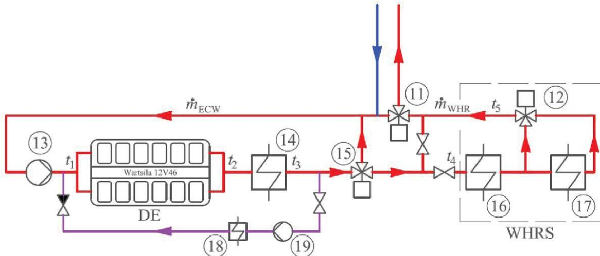
Figure 2: Diesel engine HT fresh water cooling system (Source: authors - adopted from [4], [5])
