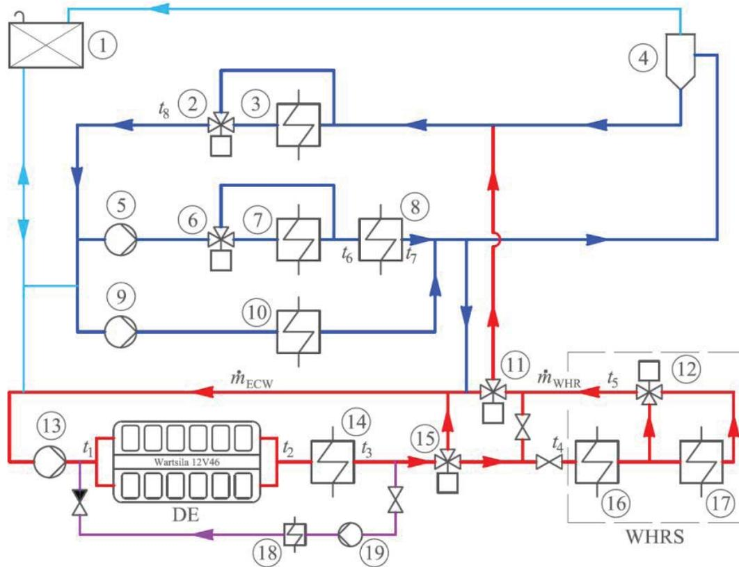
Figure 1: Diesel engine fresh water cooling system (Source: authors - adopted from [4], [5])
